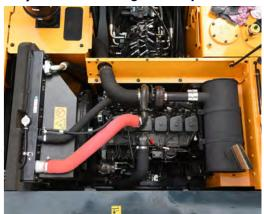
The cooling system is provided for optimum operation, guaranteeing longer life for the engine and hydraulic components. Servicing of the engine and hydraulics is considerably simplified due to total accessibility.
